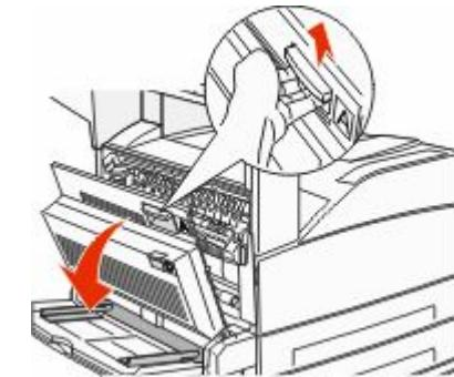
**CAUTION—HOT SURFACE:** The inside of the printer might be hot. To reduce the risk of injury from a hot component, allow the surface to cool before touching.
