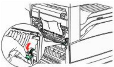
**Note:** If the jam does not move immediately, stop pulling. Push down and pull the green lever to make it easier to remove the jam. Make sure all paper fragments are removed.
