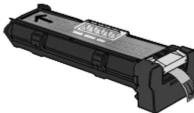
6 Align and insert the end of the photoconductor.
