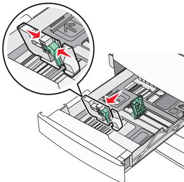
**3** Squeeze and then slide the length guide to the correct position for the paper size loaded.
