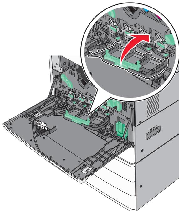
**11** Rotate the release lever clockwise to lock the cover.
