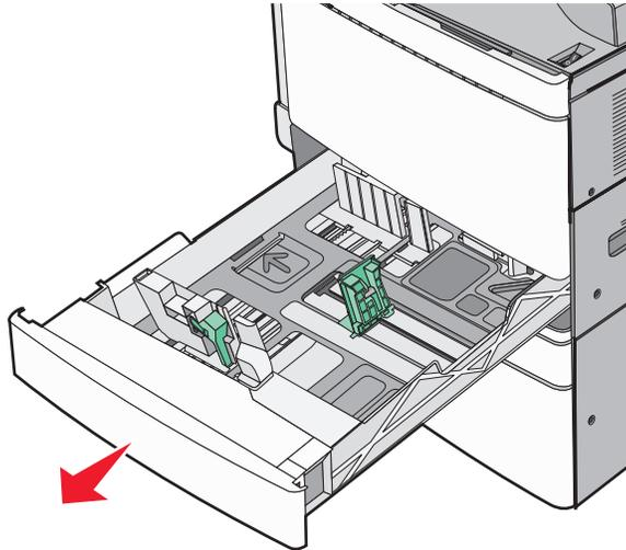
Notice the size indicators at the bottom of the tray. Use these indicators to help position the length and width guides.
