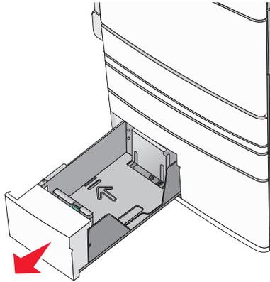
**2** Squeeze and then slide the length guide to the correct position for the paper size you are loading.
