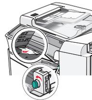
**Note:** If the paper jam on the right is difficult to remove, then rotate the knob counterclockwise.
