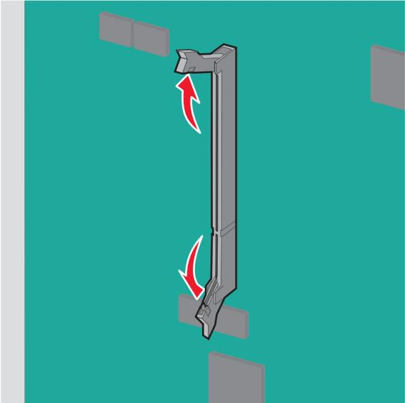
**4** Align the notch on the memory card to the ridge on the connector.
