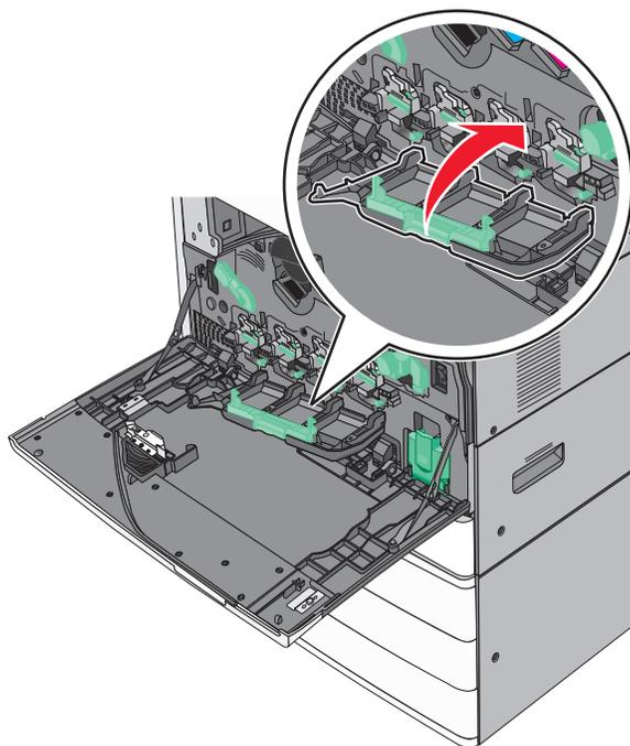
**12** Rotate the release lever clockwise to lock the cover.
