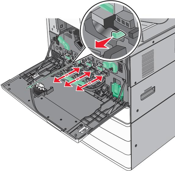
**9** Slide the printhead wipers back into place.
