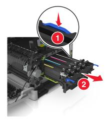
8 Remove the used developer unit.
