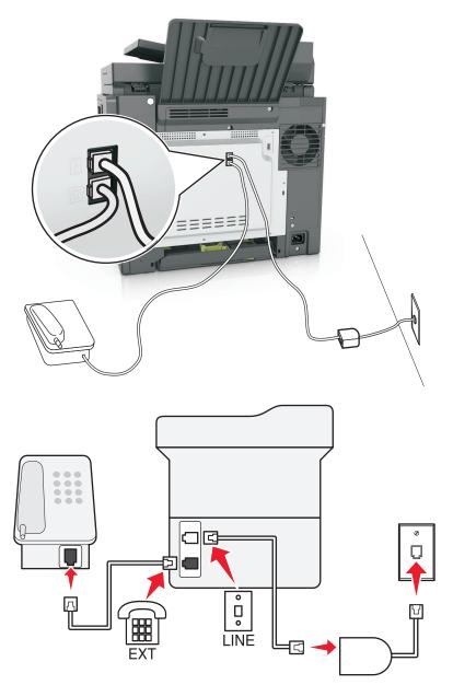
A Digital Subscriber Line splits your regular telephone line into two channels: voice and Internet. Telephone and fax signals travel through the voice channel, and Internet signals pass through the other channel. This way, you can use the same line for analog voice calls (including faxes) and digital Internet access.
