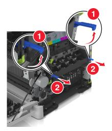
7 Press down the blue lever, and then grasp the green handles on the sides to pull out the imaging kit.
