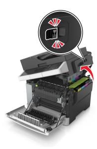
**3** Remove the toner cartridges by lifting the handles, and then gently pulling them away from the imaging kit.
