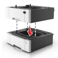
**4** Align the printer with the 650-sheet duo tray, and then lower the printer into place.
