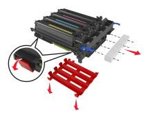
**Warning—Potential Damage:** Do not touch the shiny photoconductor drum under the imaging kit. Doing so may affect the quality of future print jobs.
