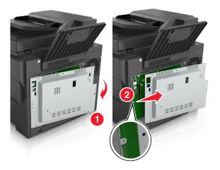
**3** Locate the appropriate connector on the controller board.
