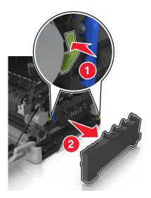
**6** Lift the blue levers on the imaging kit, and then pull the imaging kit until it stops.
