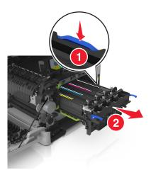
**8** Remove the used developer unit.
