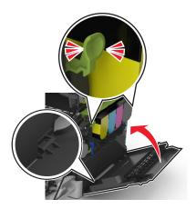
**9** Slide and hold the release latch on the right side of the printer, and then slowly close the top door.
