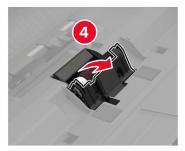
Remove the ADF separator roller.
