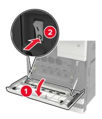
**2** Remove the ADF separator pad.
