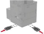
**22** Connect the 2 x 500- or 2500-sheet tray connector to the printer.
