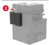
**5** Remove the controller board access cover.
