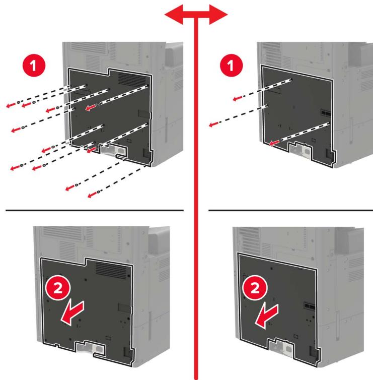
**6 移除控制器板挡板。**
