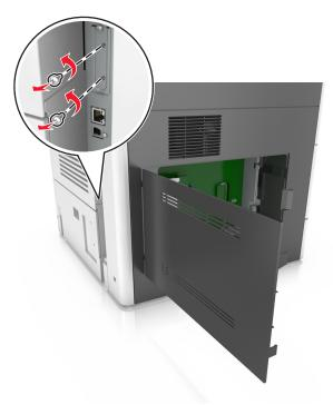
**4** Remove the printer hard disk.
