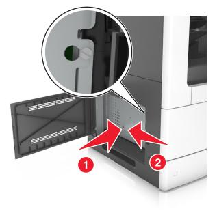
**6** Tighten the screws on the shield.
