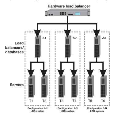
Each system group contains two identical LDD systems. Jobs are balanced between these systems in each group by the hardware load balancer or GSS. If a failure occurs in one system in a group, then the other system in the group receives all incoming jobs until the failed system can be restored.
