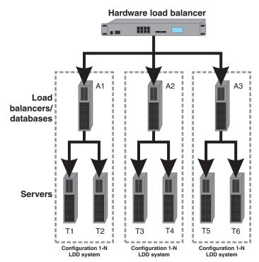
Each system group contains two identical Lexmark Document Distributor systems. Jobs are balanced between these systems in each group by the hardware load balancer or GSS. If a failure occurs in one system in a group, then the other system in the group receives all incoming jobs until the failed system can be restored.
