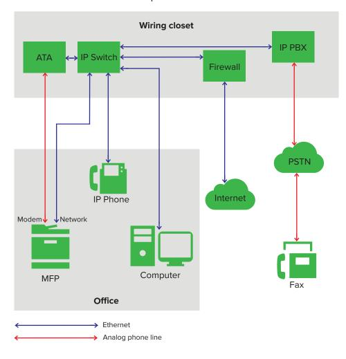
The application lets MFPs send fax data that is formatted to T.38 protocol to an IP PBX using a single network connection.
