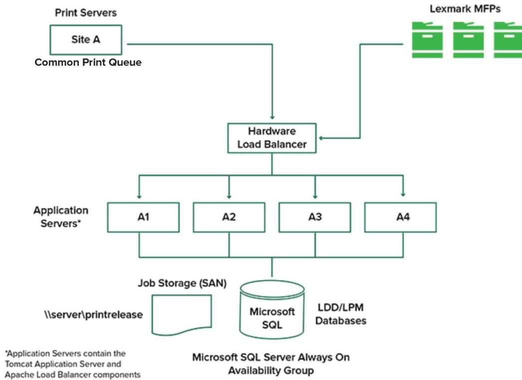
The following shows a sample diagram for achieving automated failover or redundancy using two data centers:
