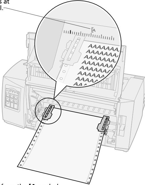
The distance from the **[A]** symbol to the left edge of the paper determines the width of the left margin.
