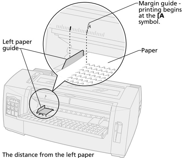
The distance from the left paper guide to the **[A]** symbol determines the width of the left margin.
