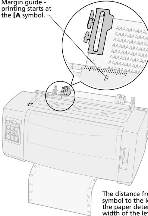
The distance from the **[A]** symbol to the left edge of the paper determines the width of the left margin.
