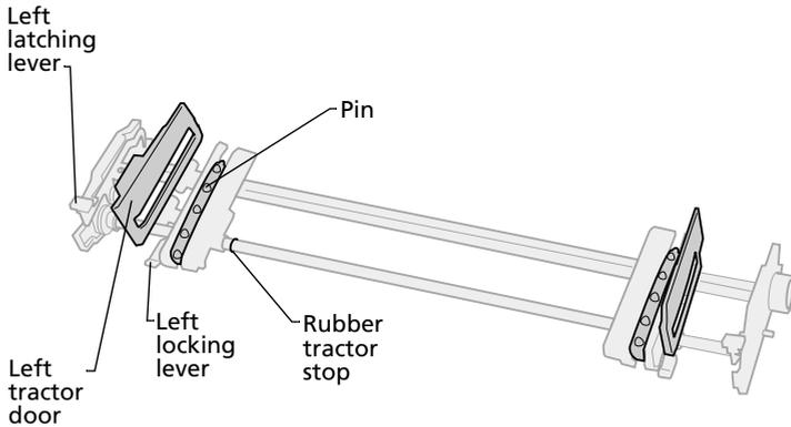
You can install the tractor unit in the push tractor position or the pull tractor position. To view an illustration of the tractor positions and paper paths available, see "Paper paths for the push tractor" on page 47.
