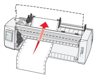
Push or pull the paper through the paper path until it passes the printhead.
