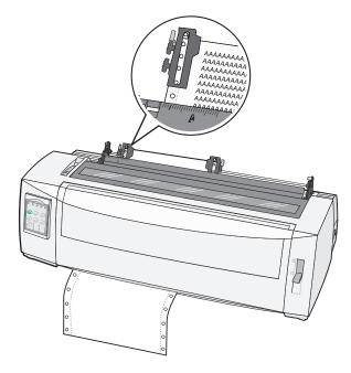
Note: The distance from the [A symbol to the left edge of the paper determines the width of the left margin.
