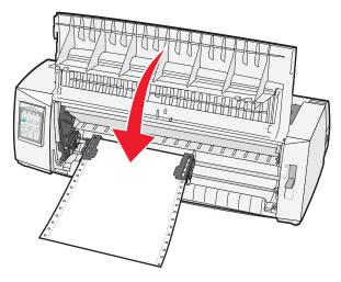
**13** Press **Start/Stop** to load the paper to Top-Of-Form and put the printer online.
