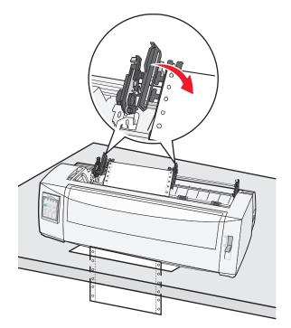
If necessary, move the left or right tractor to adjust the tractors to the paper width.
