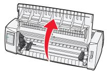
**4** Hold down the latching levers while you lift and pull the tractor unit out of the printer.
