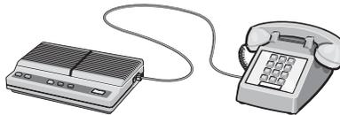
**5** Connect a third telephone cord from the answering machine to the EXT port
