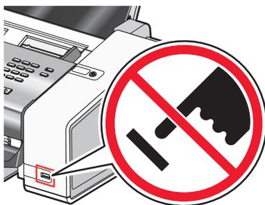
**Warning:** Do not touch the USB cable, any network adapter, or the printer in the area shown while actively printing from a PictBridge-enabled digital camera. A loss of data can occur. Also, do not remove the USB cable or network adapter while actively printing from a PictBridge-enabled digital camera.
