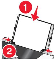
**Note:** To avoid paper jams, make sure the paper does not buckle when you adjust the paper guides.
