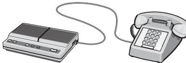
**5** Connect a third telephone cord from the answering machine to the EXT port
