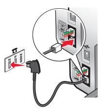
**4** If you would like to use the same line for both fax and telephone communication, connect a second telephone line (not provided) between the telephone and the F slot of an active telephone wall jack.
