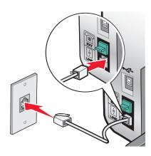
**3** Remove the protective plug from the EXT port  $\widehat{\mathbb{H}}$  of the printer.
