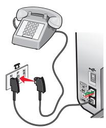
**5** If you would like to use the same line for recording messages on your answering machine, connect a second telephone line (not provided) between the answering machine and the other N slot of the telephone wall jack.
