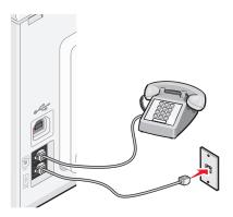
**Warning—Potential Damage:** Do not touch cables or the printer in the area shown while actively sending or receiving a fax.
