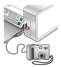
**Warning—Potential Damage:** Do not touch the USB cable, any network adapter, or the printer in the area shown while actively printing from a PictBridge-enabled digital camera. A loss of data can occur. Also, do not remove the USB cable or network adapter while actively printing from a PictBridge-enabled digital camera.
