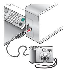
The message PictBridge camera detected. Press  $\checkmark$  to change settings. appears on the display.
