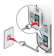
**3** Remove the protective plug from the EXT port  $\stackrel{\frown}{=}$  of the printer.
