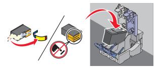
**Warning—Potential Damage:** Do *not* touch the gold contact area on the back or the metal nozzles on the bottom of the cartridge.
