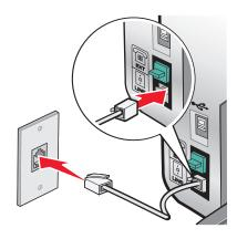
**3** Remove the protective plug from the EXT port  $\widehat{\mathbb{H}}$  of the printer.
