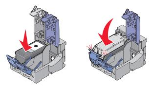
**5** Remove the tape from the back and bottom of the color cartridge, and insert the cartridge in the right carrier.
