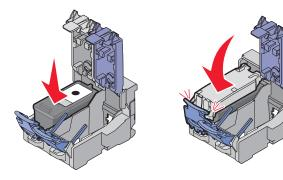
Remove the tape from the color cartridge, and then insert the cartridge in the right carrier.
