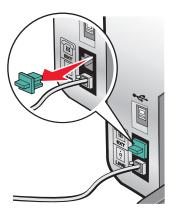
**4** Connect the other telephone cord to a telephone, and then plug it into the EXT port of the printer.
