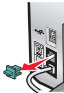
**Note:** Once this plug is removed, any country- or region-specific equipment you connect to the printer by the adapter, as shown, will not function properly.
