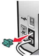
2 Connect your telecommunications equipment directly to the EXT port on the back of the printer.
