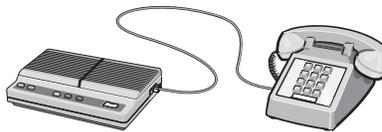
**5** Connect a third telephone cord from the answering machine to the EXT port
