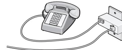
2 Connect your telecommunications equipment directly to the EXT port on the back of the printer.
