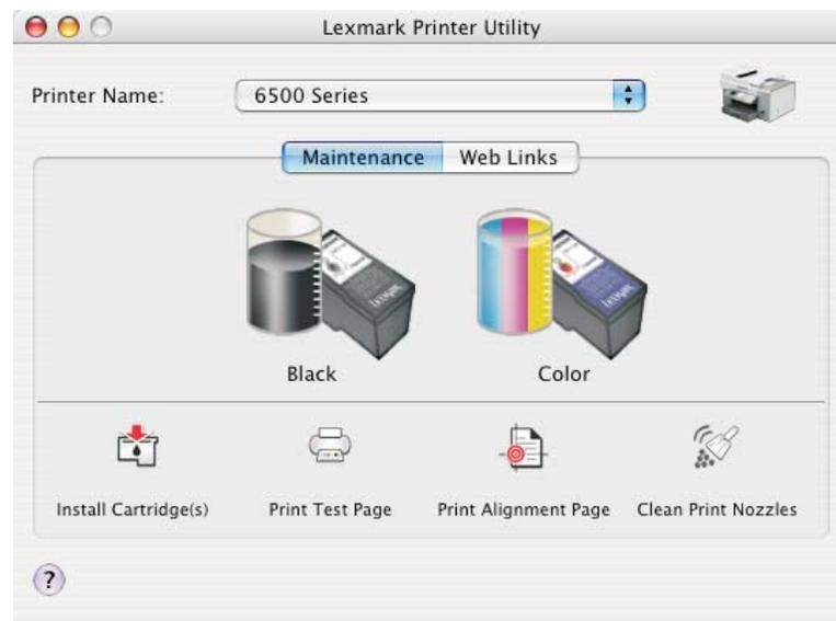
If an exclamation point (!) appears on a cartridge, the ink level is low. Install a new cartridge. For more information, see “Installing print cartridges” on page 133.
