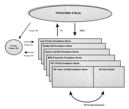
The SEM command is used to temporarily switch the printer emulation mode. It also resets the margins and other parameters.
