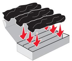
6 Close the box to protect the photoconductor units from light exposure.
