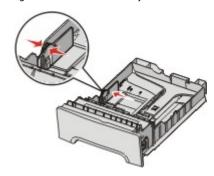
3 Squeeze the length guide tabs together as shown, and slide the length guide to the correct position for the size of paper being loaded. Notice the size indicators in the window in the bottom of the tray. Use these indicators to help position the guide. Notice the load lines on the width guide tab: they indicate the maximum height for loading paper.
