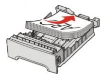
**6** Squeeze the width guide tabs, and slide the width guide to lightly touch the side of the stack.
