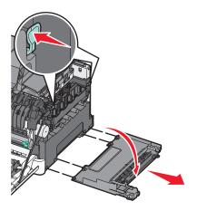
**5** Press the green levers on each side of the waste toner box, and then remove it.
