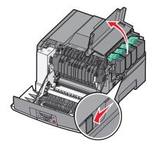
3 Remove the toner cartridges by lifting the handles and then gently pulling them away from the imaging kit.
