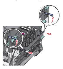
7 Press down on the blue levers, grasp the handles on the sides, and then pull the imaging kit out.
