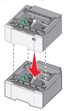
**4** Align the printer with the 650-sheet duo drawer, and then lower the printer into place.
