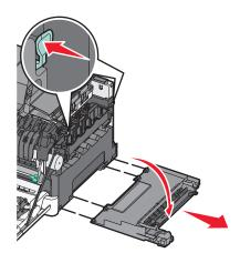
**5** Press the green levers on each side of the waste toner box, and then remove it.
