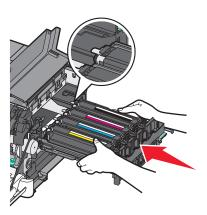
15 Gently, but firmly push the blue levers down until the imaging kit drops into place.
