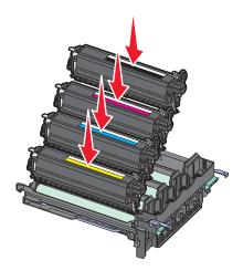
**Note:** Make sure each developer unit is inserted into a matching color slot.
