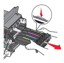
8 Remove the used developer unit.
