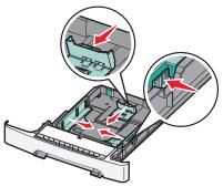
Squeeze the width guide tabs on the right guide as shown, and then slide the width guides to the sides of the tray. Notice that the two width guides move in unison when you move just the right width guide. Squeeze the length guide tabs together as shown, and then slide the length guide to the correct position for the paper size being loaded.
