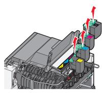
Remove the toner cartridges by lifting the handles, and then gently pulling away from the imaging kit.
