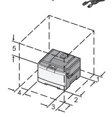
When the printer is set up, allow clearance around it as shown.
