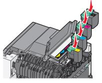
Insert the toner cartridge into the imaging kit by aligning the rollers on the toner cartridge with the tracks. Push the toner cartridge until it *clicks* into place.
