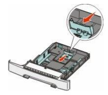
**Note:** Use the size indicators on the bottom of the tray to help position the guide.
