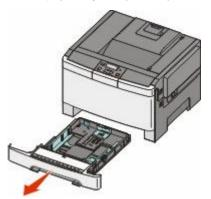
**2** Squeeze the length guide tab inward as shown, and slide the guide to the correct position for the paper size being loaded.
