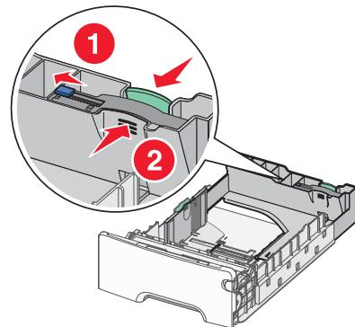
**Note:** The length guide has a locking device. To unlock the tray, slide the button on top of the length guide to the left as shown. To lock the tray once a length has been selected, slide the button back to the right.
