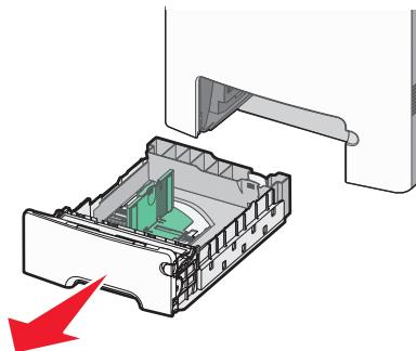
Notice the size indicators on the bottom of the tray. Use these indicators to help position the guides.
