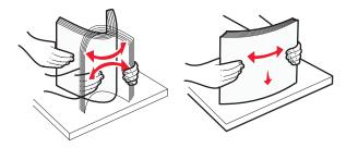
**5** Load the paper stack toward the back of the tray with the recommended printable side faceup.
