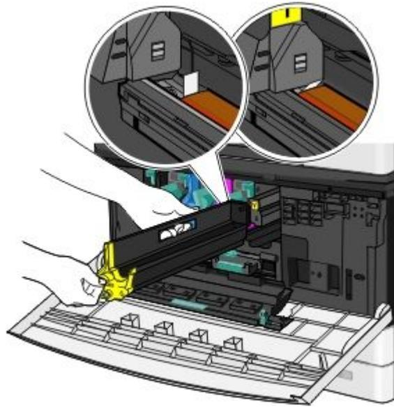
**a** Insert the imaging unit into the printer until it *clicks* into place.
