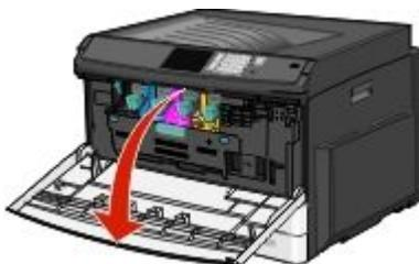
2 Turn the toner lock lever to the right and pull the toner cartridge out.
