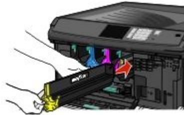
**b** Using both hands, push the sides of the internal cover firmly until the cover *clicks* into place.
