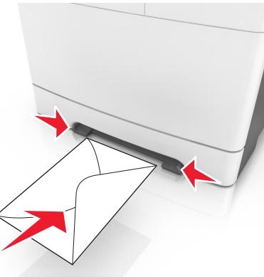
**2** Feed paper into the manual feeder only to the point where its leading edge can contact the paper guides.
