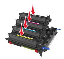
**13** Remove the red packing strip from the imaging kit.
