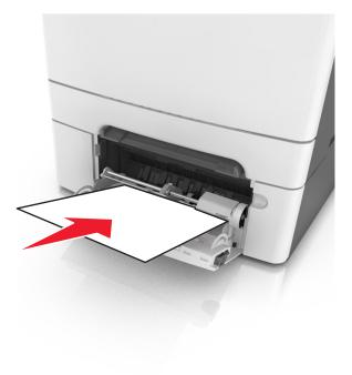
**4** Slide the paper guide until it rests lightly against the edge of the paper stack.
