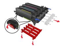
**Warning—Potential Damage:** Do not touch the shiny photoconductor drum under the imaging kit. Doing so may affect the quality of future print jobs.
