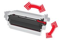
**11** Remove the red packing strip and the attached fabric from the developer units.
