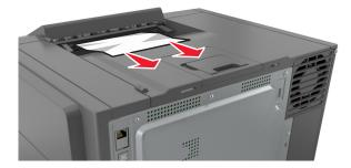
2 From the printer control panel, touch stoclear the message and continue printing. For non-touch-screen printer models, select Next > Clear the jam, press OK, and then press of to confirm.
