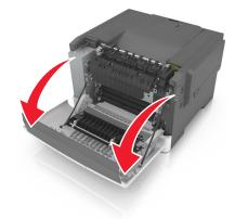
**2** Pull the green lever to open the fuser cover.
