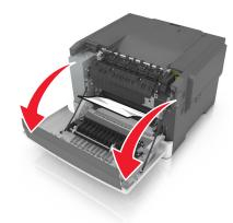
2 Firmly grasp the jammed paper on each side, and then gently pull it out.Note: Make sure all paper fragments are removed.
