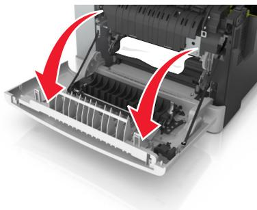
**a** If there is a jammed paper under the fuser, then firmly grasp the paper on each side, and then gently pull it out.
