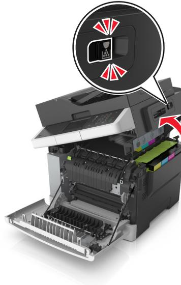
3 Pull the green lever to open the fuser cover.
