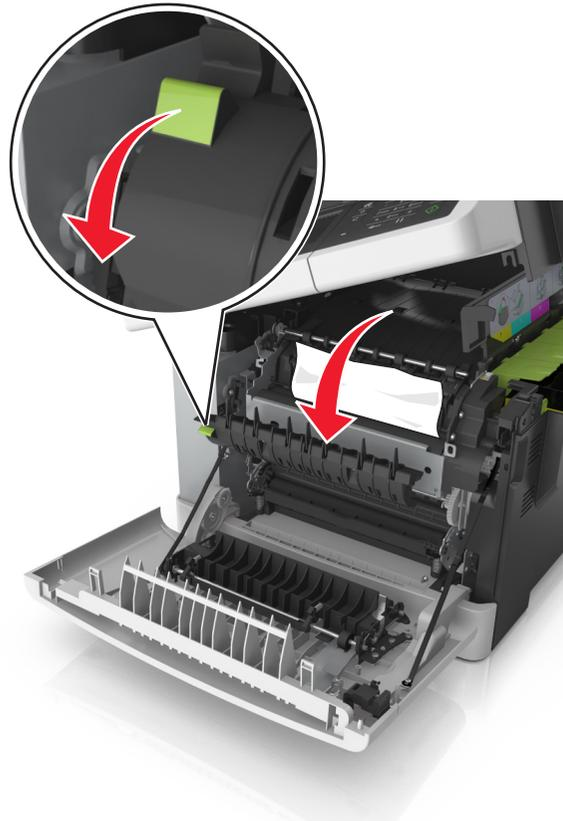
**c** If there is a jammed paper in the fuser, then hold down the fuser cover, and then remove the paper.
