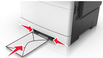
2 Feed paper into the manual feeder only to the point where its leading edge can contact the paper guides.
