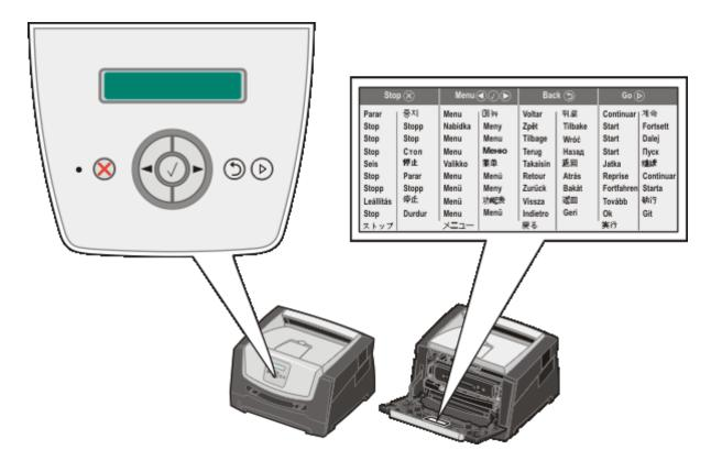
The use of the buttons and the layout of the display are described in the following table.
