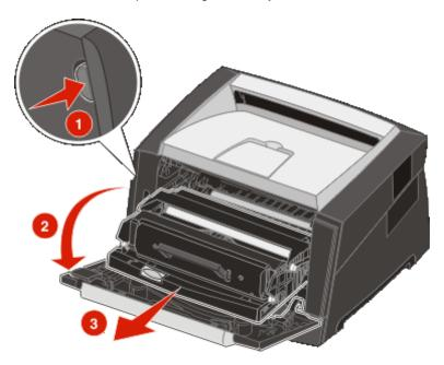
3 Lift the green flap at the front of the printer, and then remove the jammed pages beneath the flap.
