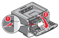
Press the door release button and lower the front door.
