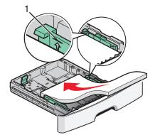
Load the paper stack toward the back on the tray as shown with the recommended print side facedown.
