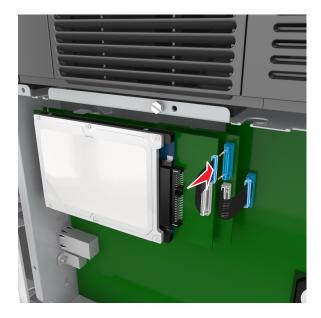
4 Align the standoffs of the printer hard disk to the holes in the controller board cage, and then press the printer hard disk down until the standoffs are in place.
