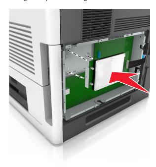
**Note:** Make sure the cables are neatly tucked under the printer hard disk.
