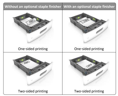
• If you are loading prepunched paper for use with the staple finisher, then make sure the holes on the long edge of the paper are on the right side of the tray.
