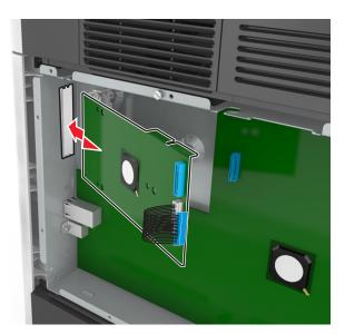
**Note:** Hold the ISP at an angle over the plastic bracket so that any overhanging connectors will pass through the ISP opening in the controller board cage.
