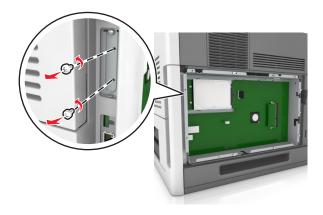
4 Remove the printer hard disk.
