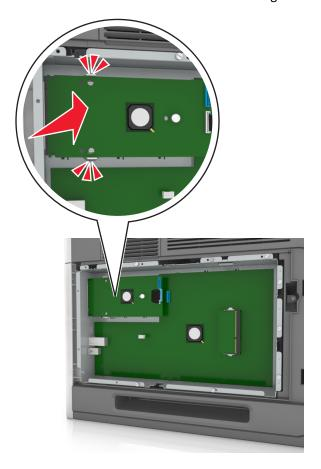
**8** Use the provided thumbscrew for the ISP to attach the plastic bracket to the ISP.
