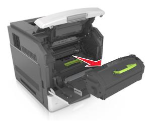
**3** Lift the green handle, and then pull out the imaging unit from the printer.
