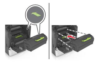
**Warning—Potential Damage:** When replacing a toner cartridge, do not leave the imaging unit exposed to direct light for an extended period of time. Extended exposure to light may cause print quality problems.
