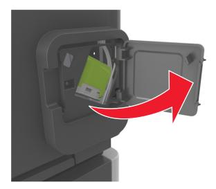
**2** Pull down the latch of the staple cartridge holder, and then pull the holder out of the finisher.
