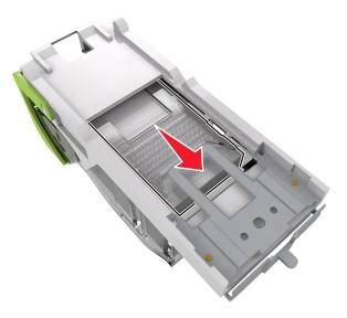
**Note:** If the staples are at the rear of the cartridge, then shake the cartridge downward to bring the staples near the metal bracket.
