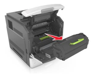
**3** Unpack the new toner cartridge, then remove the packing material, and then shake the cartridge to redistribute the toner.
