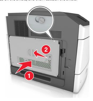
**6** Tighten the screws on the shield.
