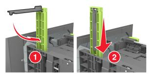
**d** Squeeze the length guide and slide it to the correct position for the size of the paper being loaded until it *clicks* into place.
