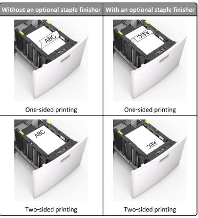
• If you are loading prepunched paper for use with the staple finisher, then make sure the holes on the long edge of the paper are on the right side of the tray.
