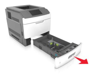
**2** Squeeze and slide the width guide to the correct position for the size of the paper being loaded until it *clicks* into place.
