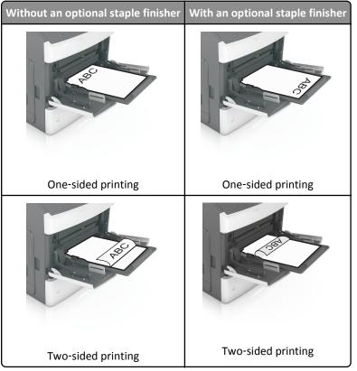
• If you are loading prepunched paper for use with the staple finisher, then make sure the holes on the long edge of the paper are on the right side of the tray.
