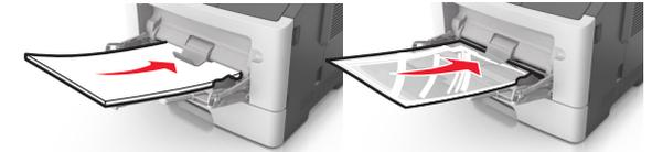
**Note:** When loading A6-size paper, make sure the multipurpose feeder extender rests lightly against the edge of the paper so that the last few sheets of paper remain in place.
