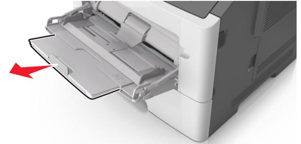
b Pull the extender gently so that the multipurpose feeder is fully extended and open.
