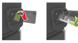
**4** Use the metal tab to lift the staple guard, and then remove any loose staples.
