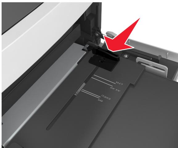
**Note:** Use the paper size indicators on the bottom of the tray to help position the guides.
