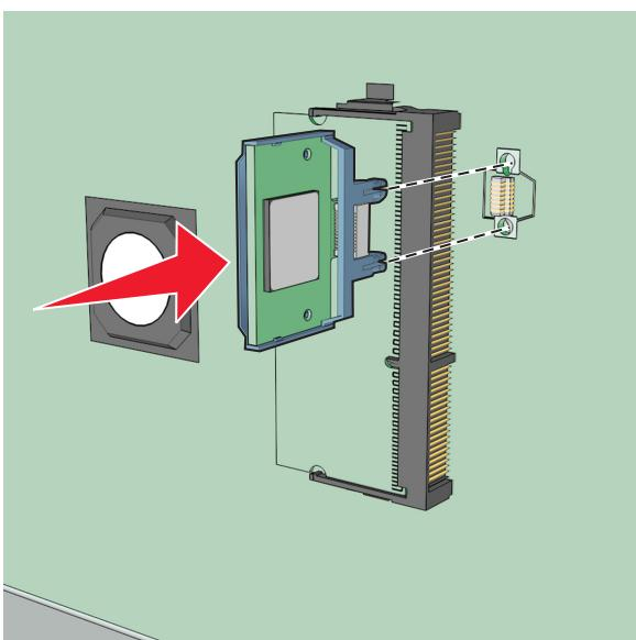
Holding the card by its sides, align the plastic pins on the card with the holes on the system board, and then push the card firmly into place.
