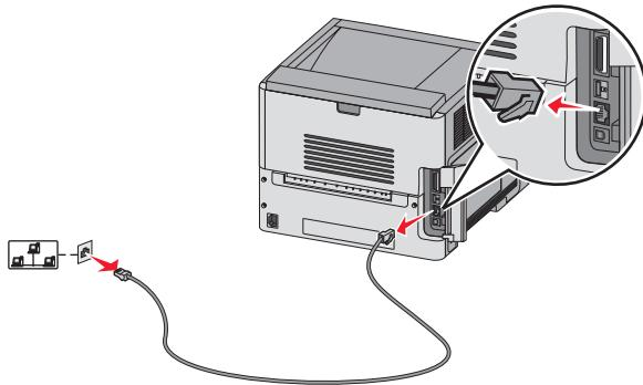
Unplug the Ethernet cable from the printer and from the router or wall outlet.
