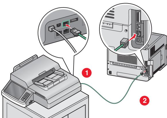
Connect the green Ethernet cable to the scanner, and then to the printer.
