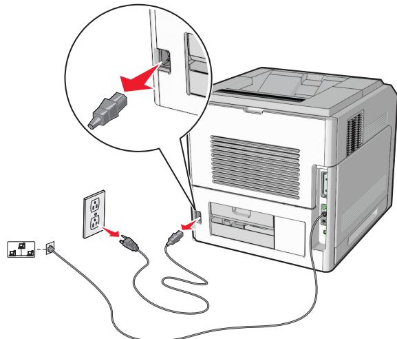
Unplug the power cord from the printer and from the wall outlet.
