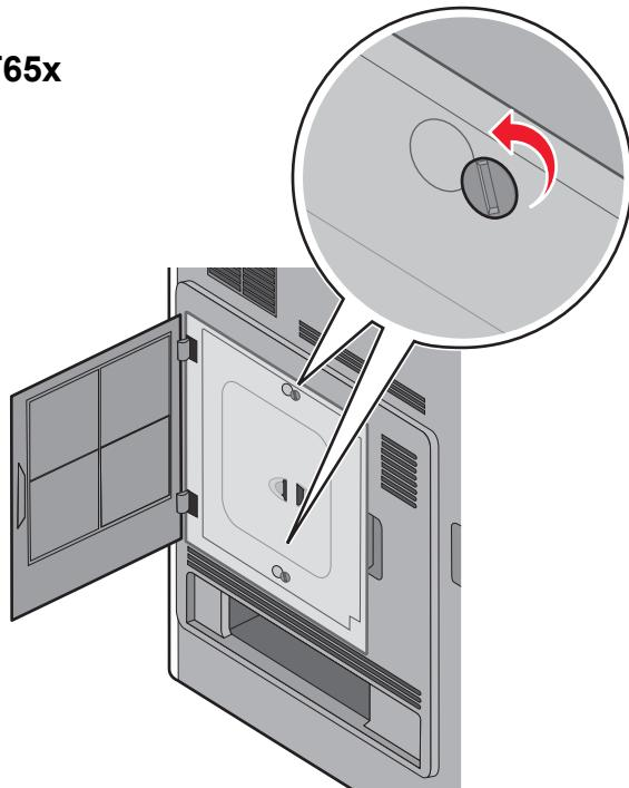
Using a flathead screwdriver, loosen the screws on the system board cover, but do not remove them.
