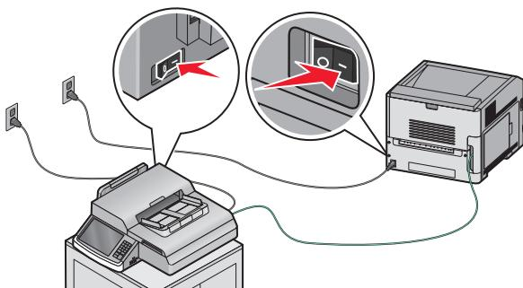
Turn the scanner on, and then turn on the printer.
