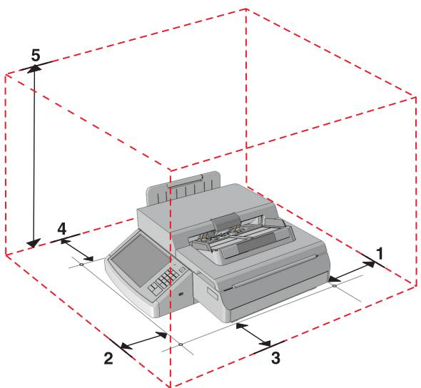
Follow this recommended amount of space around the scanner for proper ventilation.
