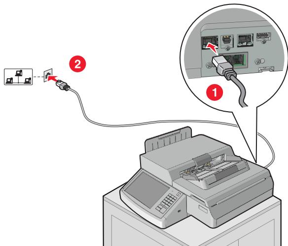
Connect the gray Ethernet cable to the scanner, and then to a router or wall outlet.
