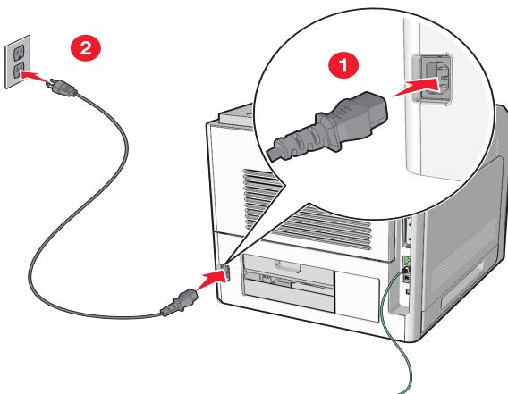
Connect the power cord to the printer, and then to a properly grounded electrical outlet that is near the product and easily accessible.
