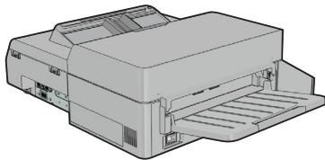
Install the exit tray to the scanner. To install the tray, align the pins on the tray to the holes on the scanner, and then *snap* the tray into place.
