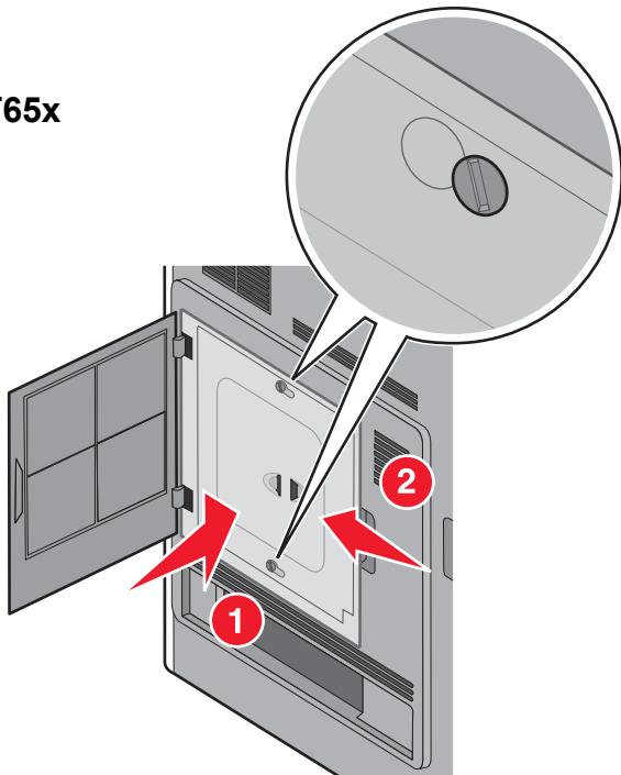
Align the screws with the holes on the system board cover, and then reattach the system board cover.
