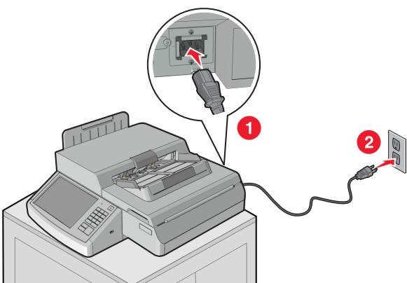
Connect the power cord to the scanner, and then to a properly grounded electrical outlet that is near the product and easily accessible.
