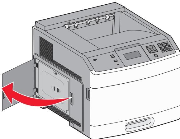
Open or remove the system board access door.
