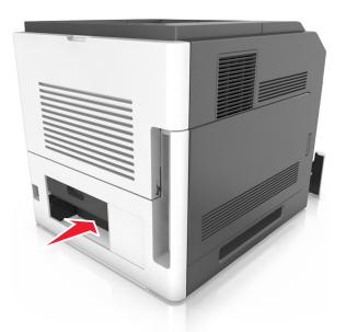
**5** Press down the rear duplex flap, then firmly grasp the jammed paper, and then gently pull out the paper.
