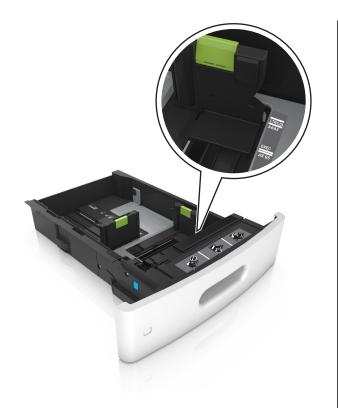
**3** Unlock the length guide, then squeeze, and then slide the guide to the correct position for the size of the paper being loaded.
