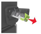
**4** Use the metal tab to lift the staple guard, and then remove any loose staples.
