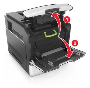
**2** Lift the green handle, and then pull out the toner cartridge from the printer.
