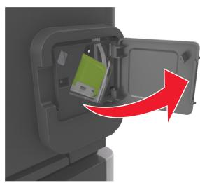
**3** Pull down the latch of the staple cartridge holder, and then pull out the holder from the printer.
