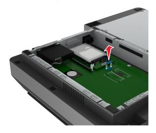
**b** Remove the screws that secure the hard disk in place.
