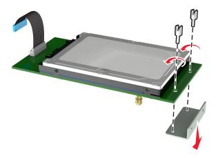
**9** Attach the small bracket to the hard disk.
