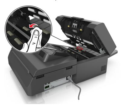
**b** To clean the rollers that rotate freely, wipe the rollers until all residue is removed.
