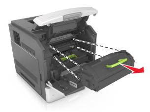
**3** Pull the imaging unit out of the printer using the handle.
