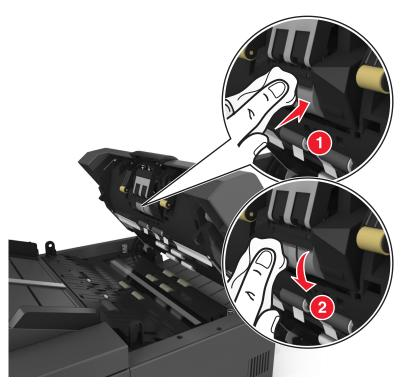
**b** To clean the rollers that rotate freely, wipe the rollers until all residue is removed.
