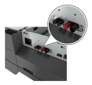
7 Insert the plug of the ISP interface cable into the connector of the system board.
