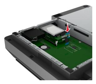
**12** Secure the hard disk to the system board cage.
