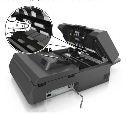
**5** Using the cleaning cloth, wipe the rollers in the lower portion of the ADF until all residue is removed.
