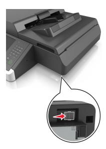
Tape the scanner cover to secure it in place.
