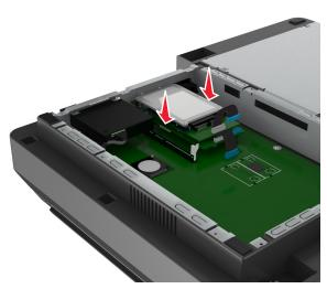
11 Insert the plug of the hard disk interface cable into the connector on the ISP.
