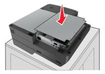
Attach all the screws to secure the system board cover.
