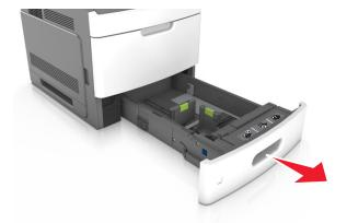
**2** Squeeze, and then slide the width guide to the correct position for the size of the paper being loaded until it *clicks* into place.
