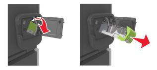
Use the metal tab to lift the staple guard, and then remove any loose staples.
