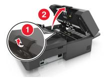
Using the cleaning cloth, wipe the rollers in the upper portion of the ADF until all residue is removed.
