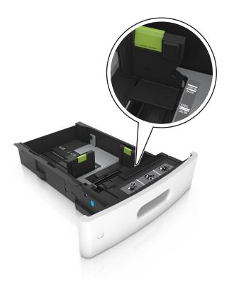
**3** Unlock the length guide, then squeeze, and then slide the guide to the correct position for the size of the paper being loaded.
