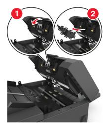
**3** Unpack the new separator pad, and then install it in the scanner.
