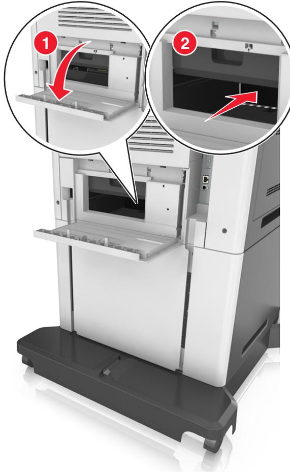
5 Press down the rear duplex flap, then firmly grasp the jammed paper, and then gently pull the paper out.
