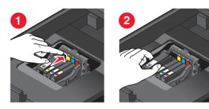
**4** Remove the ink cartridge from the pack, and then remove the protective cap from the ink cartridge. If your ink cartridge comes with a muzzle cap, then remove the cap.
