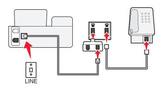
If the additional device (telephone or answering machine) has an RJ-11 connector, then you can remove the wrap plug and plug the device into the  $\stackrel{\text{\tiny [II]}}{}$  port of the printer.
