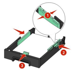
**Note:** Make sure the paper is below the maximum fill line located on the edge of the paper tray. Overloading the tray can cause paper jams.
