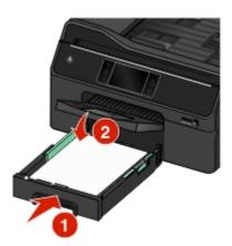
**Note:** If you extended the tray to accommodate legal-size paper, then the tray sticks out from the front of the printer when inserted.
