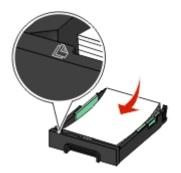
**5** Adjust the paper guides to rest against the left, right, and bottom edges of the paper.
