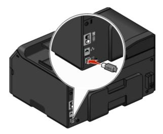
**3** Firmly plug the rectangular end of the USB cable into the USB port of the computer.
