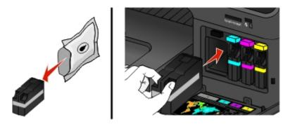
**Note:** Install the new ink cartridges immediately after removing them from the packaging to avoid exposing the ink to air.
