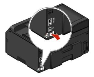
2 Firmly plug the square end of the USB cable into the back of the printer.
