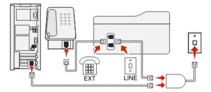
A Digital Subscriber Line splits your regular telephone line into two channels: voice and Internet. Telephone and fax signals travel through the voice channel, and Internet signals pass through the other channel. This way, you can use the same line for analog voice calls (including faxes) and digital Internet access.
