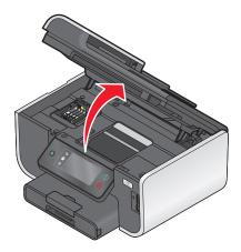
**Note:** The printhead moves to the cartridge installation position.
