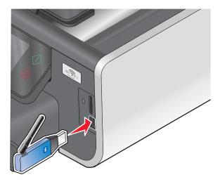
Bluetooth Dongle Connected appears on the display.
