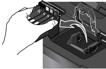
**Warning—Potential Damage:** Do not touch the printhead nozzles.
