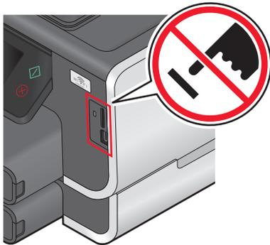
**Warning—Potential Damage:** Do not touch any cables, any network adapter, any connector, the memory device, or the printer in the areas shown while actively printing, reading, or writing from the memory card. A loss of data can occur.
