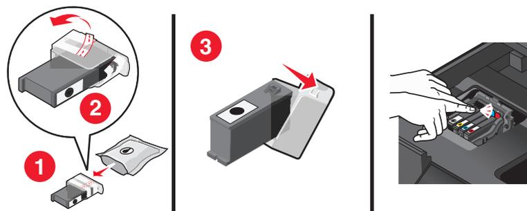
If your ink cartridge comes with a twist cap, then twist and remove the cap.
