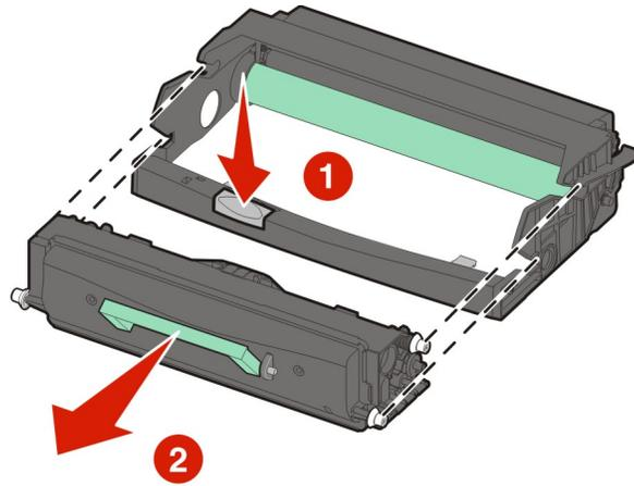
4 Unpack the new photoconductor kit. Be careful not to touch the photoconductor drum.
