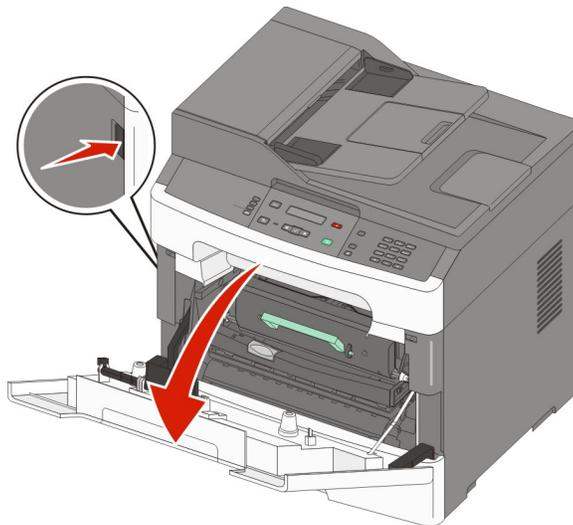
**2** Press the button on the base of the photoconductor kit, and then pull the toner cartridge out using the handle.
