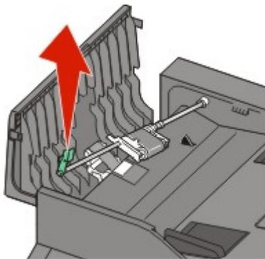
4 Use a clean, lint-free cloth dampened with water to wipe the separator roller.
