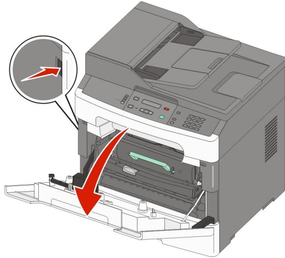
2 Pull the photoconductor kit and toner cartridge out of the printer as a unit by pulling on the toner cartridge handle.
